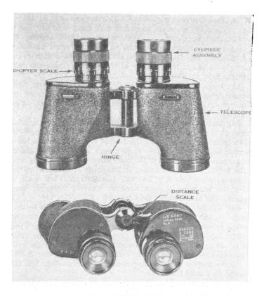
FIGURE 13.—Binocular M3.
