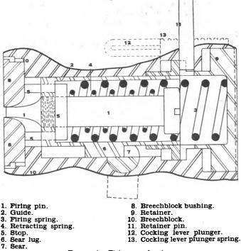
FIGURE 4.-Firing mechanism.
