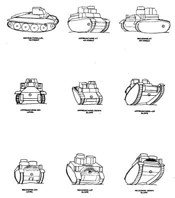
FIGURE 48.—Points of aim when engaging a moving tank. (Circle with dot in center indicates correct aiming point.)
