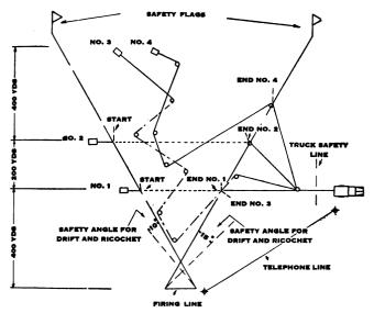
FIGURE 51.—Range for firing 37-mm ammunition at stationary or towed targets.
