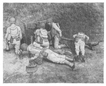
FIGURE 32 .--- Sinking trails on first round.
